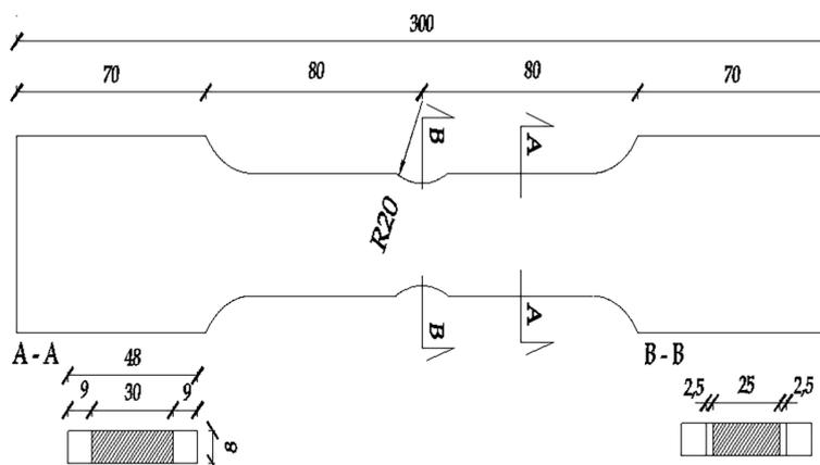
Figure 1. Scheme of a sample made of S235JR mild steel
