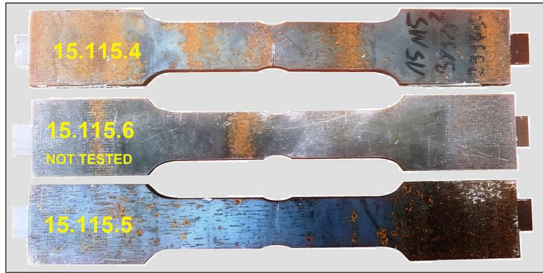
**Figure 5.** CFRP-reinforced mild steel samples subjected to fatigue load in the range  $0.15 \div 1.15 R_{eH}$
