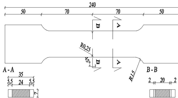
Figure 2. Scheme of a sample made of over 100-year-old steel (puddled steel)
