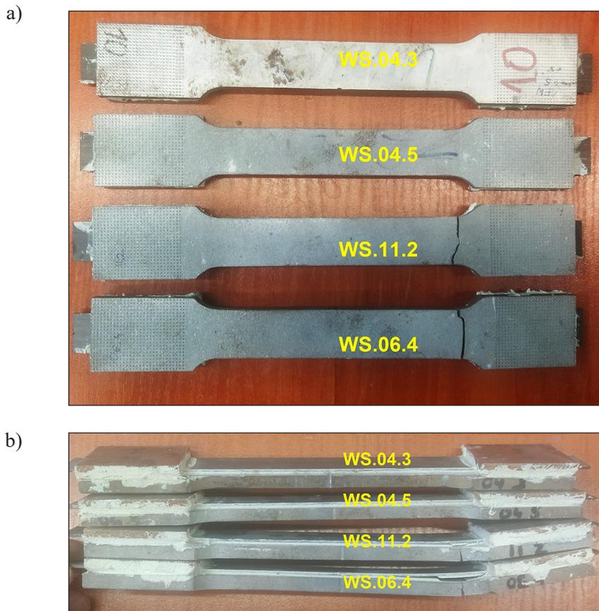
Figure 7. Damaged puddled steel samples reinforced with CFRP
