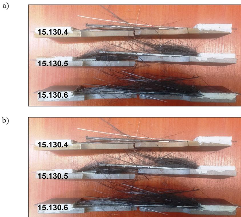
**Figure 6.** CFRP-reinforced mild steel samples subjected to fatigue load in the range  $0.15 \div 1.30 R_{eH}$
