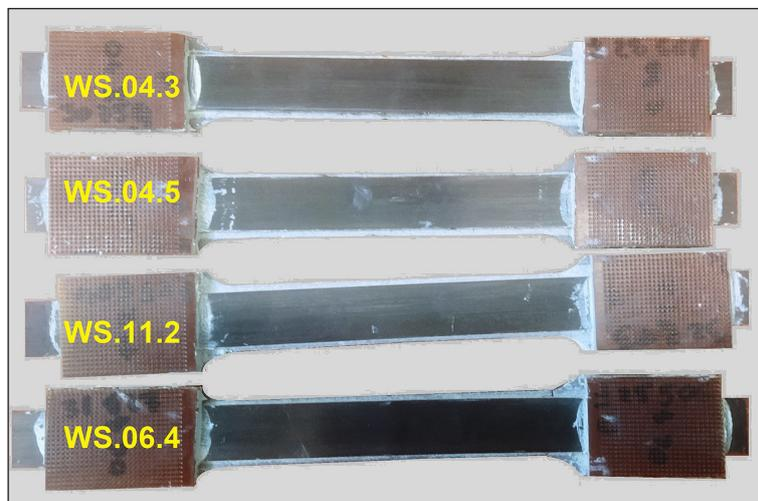
**Figure 4.** Reinforced samples made of 100-year-old steel
