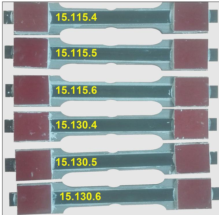
**Figure 3.** Reinforced samples made of S235JR mild steel
